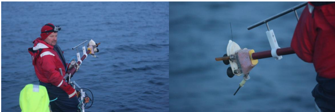
To the left the ARTS system ready for launching, and at right the LKRobotBiopsyCarrier in detail
