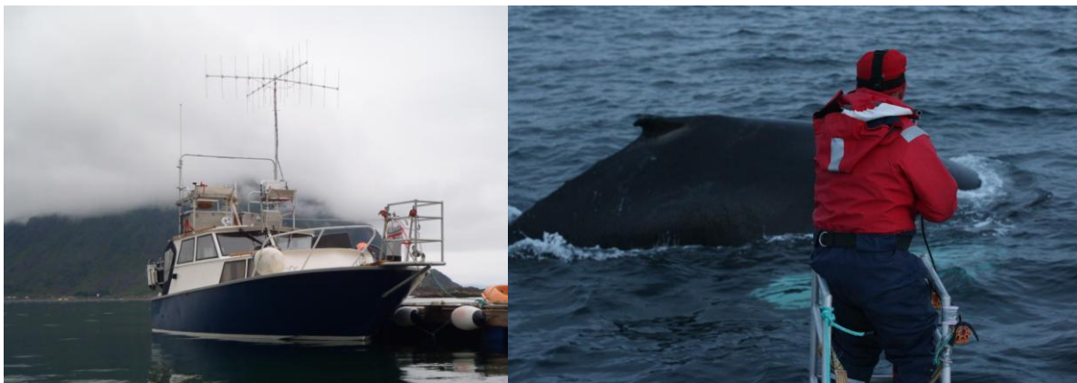
RV Blåstål with an outdoor upper bridge and a setup with Yagi antennas for tracking (left) and gunner platform (right)
